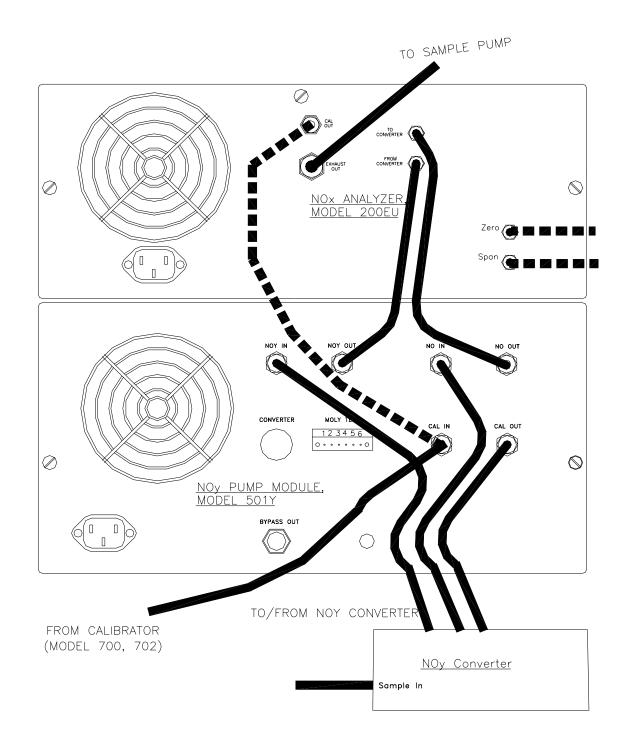
Figure 1.1 - Rear Panel Pneumatic Connections
